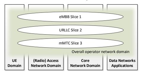
*Figure 4:* Network slicing concept with three slice types.
