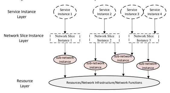
Figure 6: Network slicing concept with sub-network instances.
