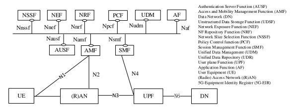
*Figure 5:* Service-based 5G architecture and defined network functions.
