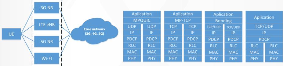
Multi-connectivity (MC) of single user terminal to multiple radio access points is a 5G key enabler in order to satisfy the demanding requirements on 5G mobile networks. Multi-connectivity supports simultaneous connectivity and aggregation across different technologies such as 5G, LTE, and unlicensed technologies such as IEEE 802.11 (Wi-Fi)
