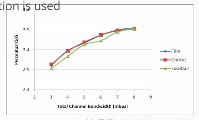
MulTCP Each stream is delivered at the same quality over the whole bit rate range
