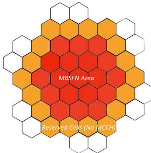
Figure 4: Example of MBSFN network with a ring of Reserved Cells.
