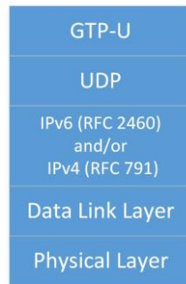
Figure 20. Transport network layer for MBMS data streams over M1 in LTE.
