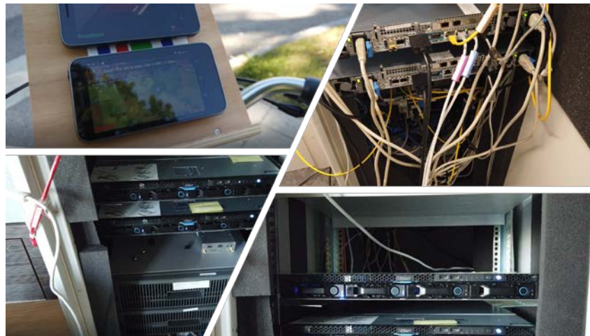
Figure 6: Equipment at the IRT premises showing the Bittium phones employed for the trials, the server that allocates the virtualized network functions of the core provided by Nokia and Expway and the base station provided by Nokia.
