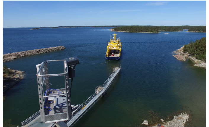
Fig. 3. The 700 MHz transmission antenna installed to a person lift at Kustavi shore.
