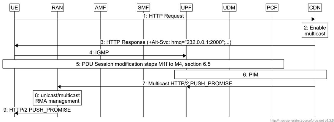
Figure 4 Dynamic delivery mode with multicast QUIC
