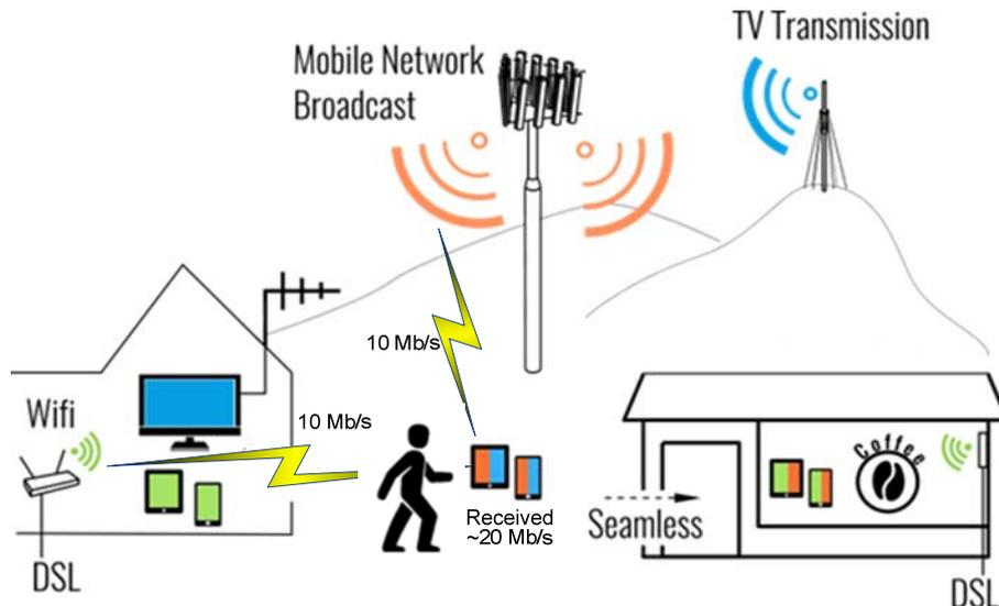
Figure 13 Multilink implementation for the bandwidth increasing
