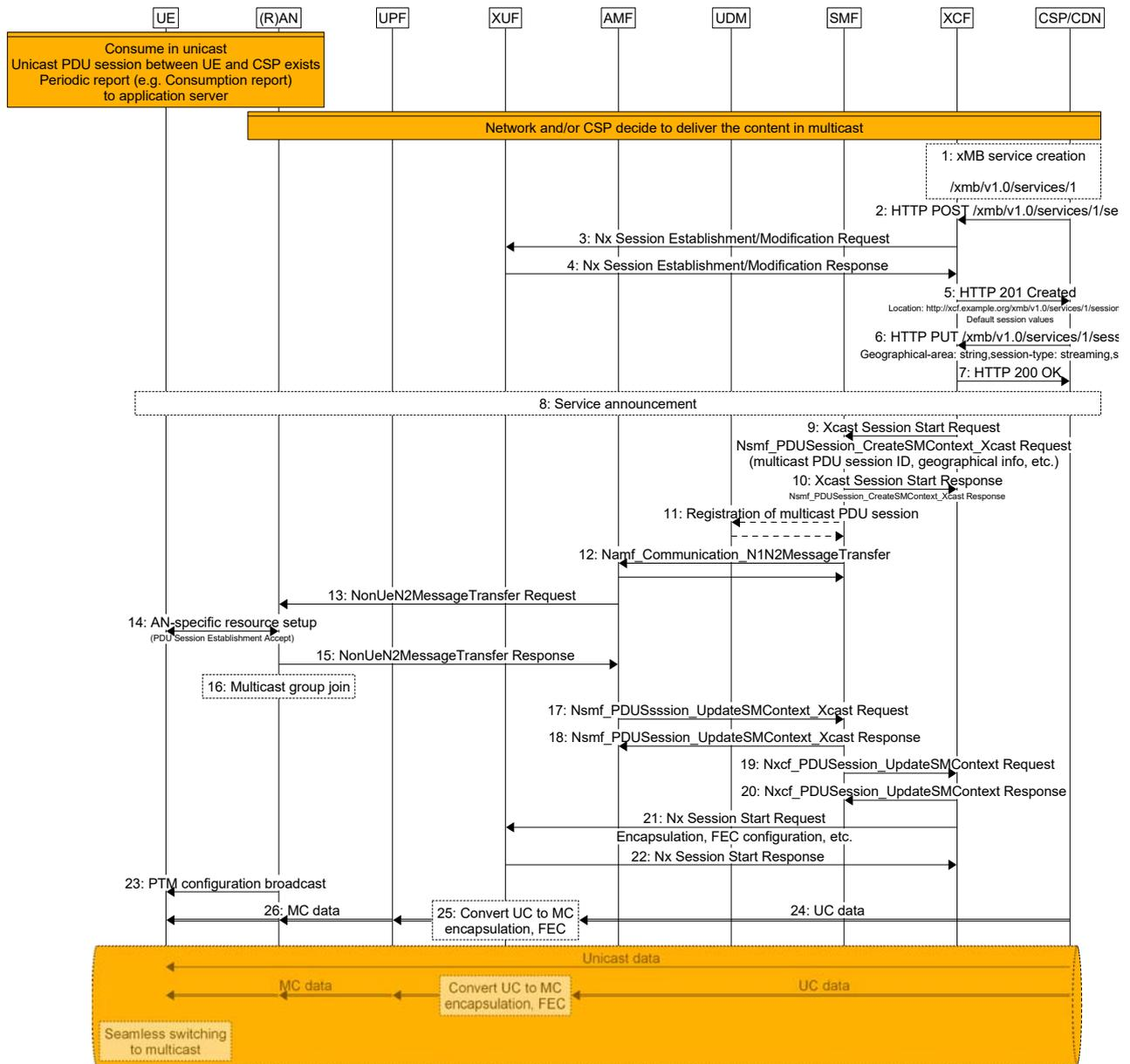
Figure 6 Dynamic delivery mode selection with point-to-multipoint services for architecture alternative 2
