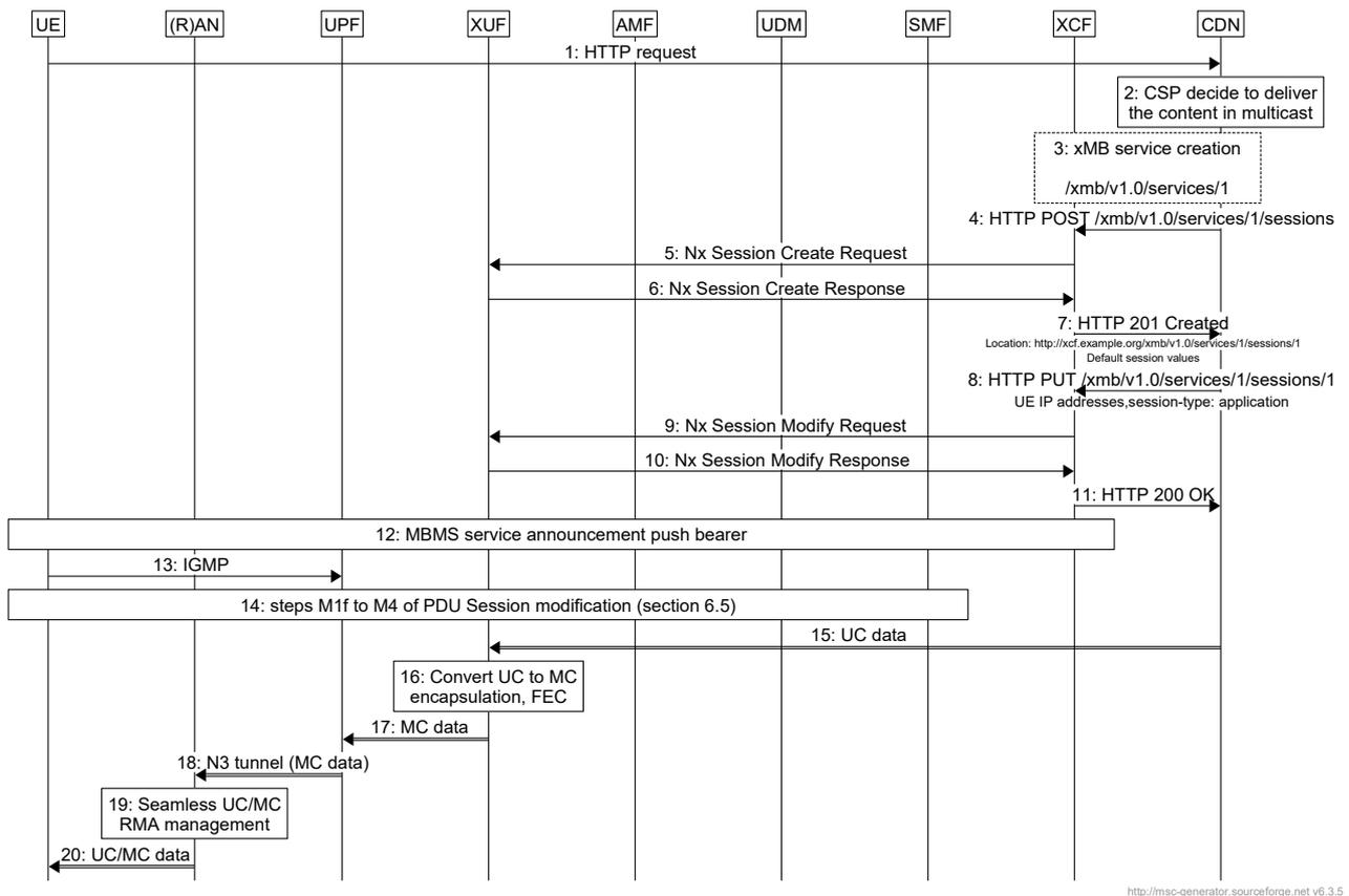
Figure 5 Dynamic delivery mode selection with point-to-multipoint services for architecture alternative 1
