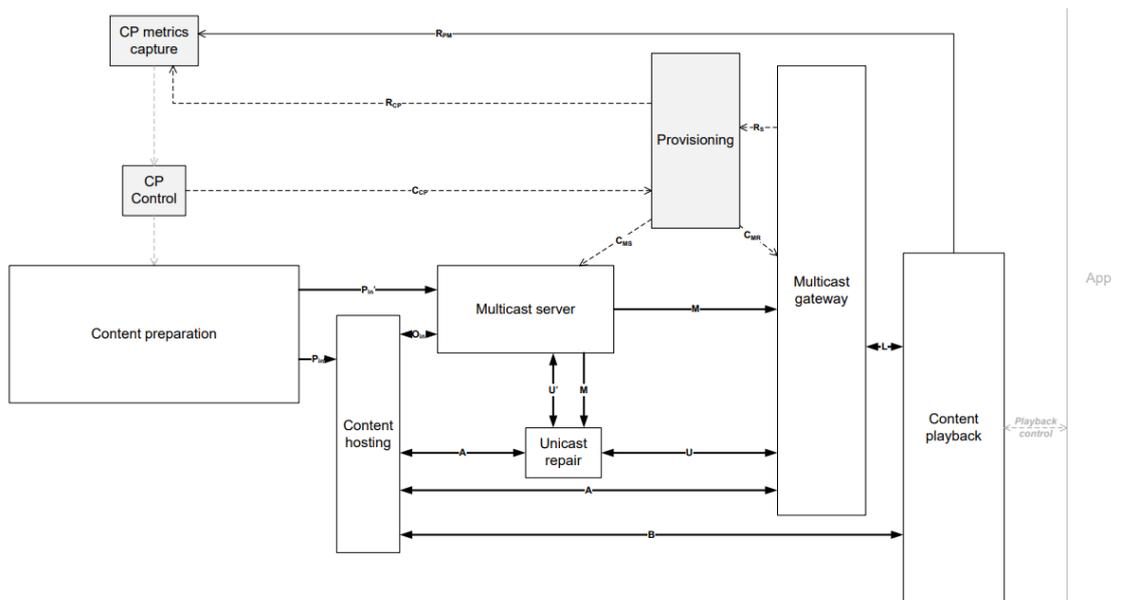
Figure 7 DVB Multicast ABR reference architecture
